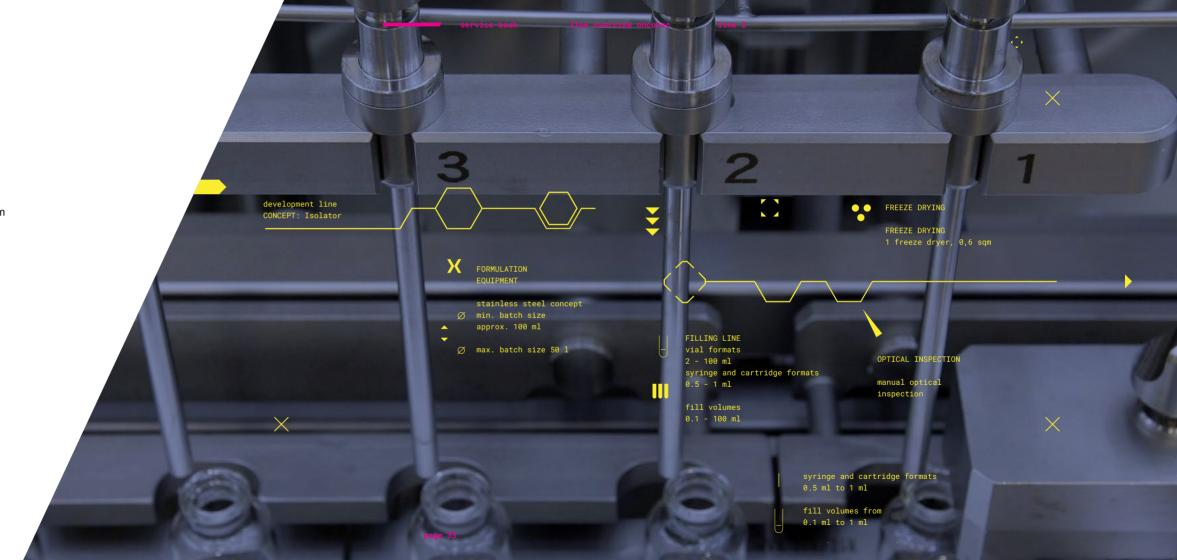
Production line 3 is an isolator filling line which allows us to produce batch sizes between 80 and 500 liters. It is equipped with two freeze dryers with shelf area of 14 sqm each. The vial fill volumes range between 6 ml and 100 ml using a time-pressure-filling system.
