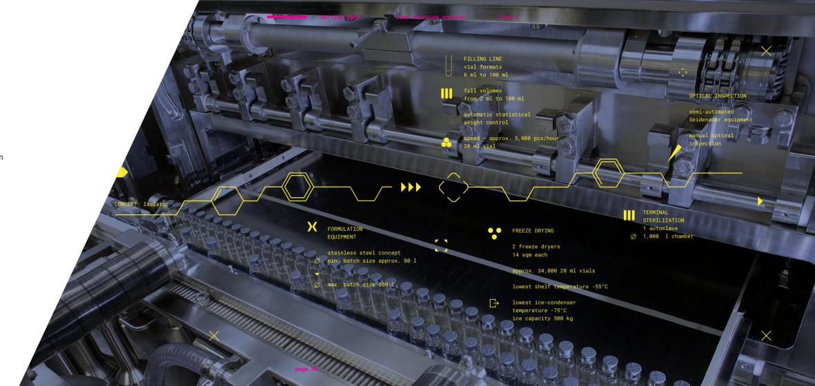
Production line 4 is an isolator line for filling of nested pre-filled syringes and cartridges. Its capacity is 50 million syringes/cartridges per year with batch sizes from 50 till 200 I, using a time-pressure filling system. The filling volumes range between 0.2 ml and 5 ml.
