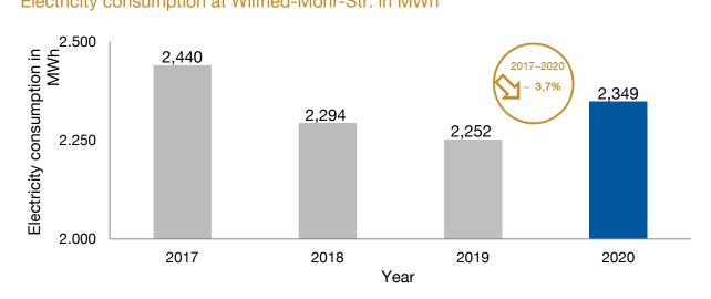
Electricity consumption at Wilfried-Mohr-Str. was reduced continuously from 2017 to 2019. This was facilitated by e.g. the LED conversion of the incoming goods and dispatch area. The increase in electricity consumption in 2020 is probably due to the installation of the PEN assembly and the two-shift system introduced because of the Corona pandemic.
