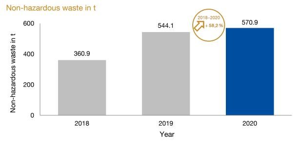
The increasing amounts of non-hazardous waste are mainly due to the accompanying increase in production. The increase of plastic waste in Tornesch by approx. 59.5 % was caused in particular by the installation of the PEN assembly as the PEN components are delivered in plastic trays and tubs.
